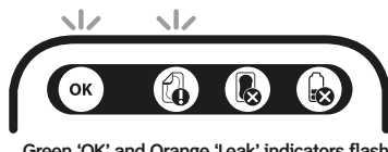
Green 'OK' and Orange 'Leak' indicators flash
